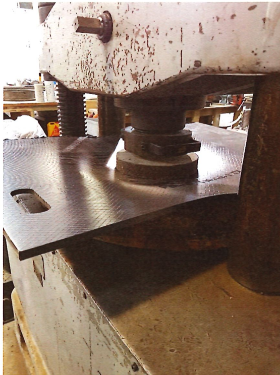
Figure 4 - After 45kN load is removed
